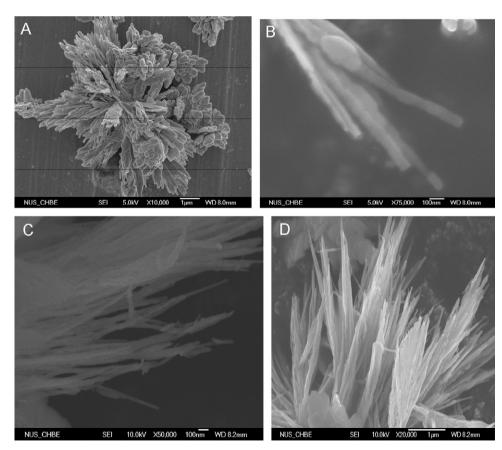
Fig. 1. FESEM images of  $La_2CuO_4$  single-crystal nanofibers (hydrothermal synthesis for 20 h). (A) Groups of highly oriented and uniform-diameter fibers; (B) an enlarged image of some individual fibers; (C) after being treated in air at 700 °C for 1 h; (D) after being tested for SRM reaction lifespan for 60 h.
