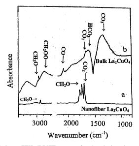
Fig. 5. In situ FTIR (DRIFT) spectra of methanol adsorption over the  $H_2$ -reduced  $La_2CuO_4$  (a) nanofibers and (b) bulk powder.
