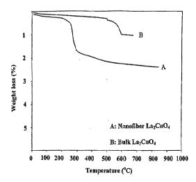
Fig. 3. Thermogravimetric (TG) curves of (A) nanofiber  $La_2CuO_4$  and (B) bulk powder  $La_2CuO_4$  in a  $H_2$  flow.
