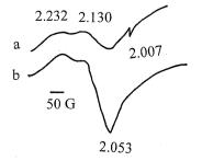
Fig. 4. EPR spectra of  $H_2$ -reduced  $La_2CuO_4$  (a) nanofibers and (b) bulk powder.
