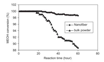
Fig. 2. Methanol conversions as a function of time-on-stream over ( $\blacklozenge$ ) nanofiber La<sub>2</sub>CuO<sub>4</sub> catalyst at 250 °C and ( $\blacktriangle$ ) bulk powder La<sub>2</sub>CuO<sub>4</sub> catalyst at 400 °C.
